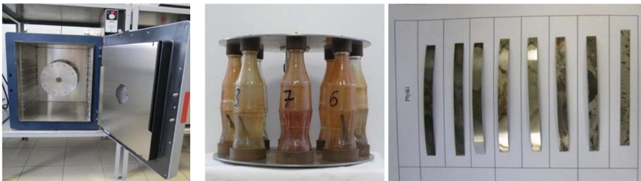
Fig. 1 Wheel test setup according to NACE ID182-2005, the rotation apparatus with testing bottles after the corrosion test, Steel plates after corrosion Wheel Test
