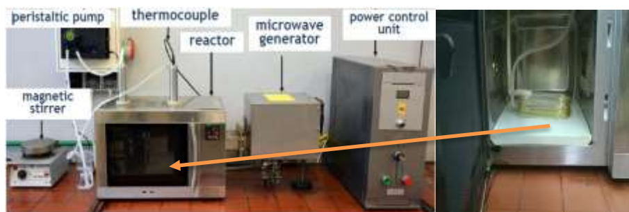
Fig. 1. Schematic view of the transesterification of rapeseed oil apparatus
